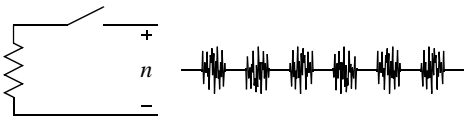
Fig. 1. The resistor generates white thermal noise. The switch opens and closes periodically, so the noise at the output is cyclostationary.
